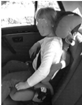
Figure 3a. The most common sagittal sitting posture using the booster seat with the large head side supports in the study by Andersson et al. 2010.
