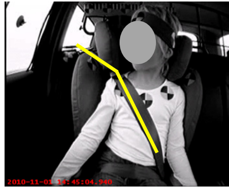
Figure 4b. Lateral inboard motion of a child during a swerving maneuver, using booster seat with backrest (Bohman et al. 2011b)
