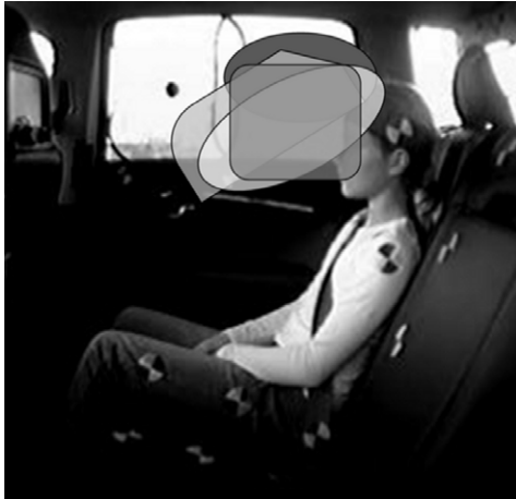
Figure. 1a. Schematic plot representing trajectories for forehead markers for child volunteers from the brake event study by Stockman et al. (2012). From darker to lighter grey, the coloured areas represent: taller children (135-150 cm) on booster cushion, taller children on vehicle seat, shorter children (107-123 cm) in booster seat with backrest and shorter children on booster cushions.
