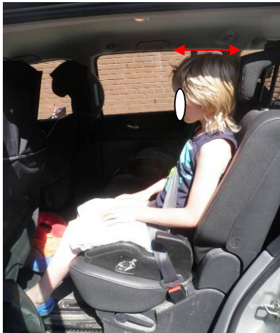
Figure 2c. Child 7 yo – 133 cm in rear seat of Renault Grand Espace using booster cushion.
