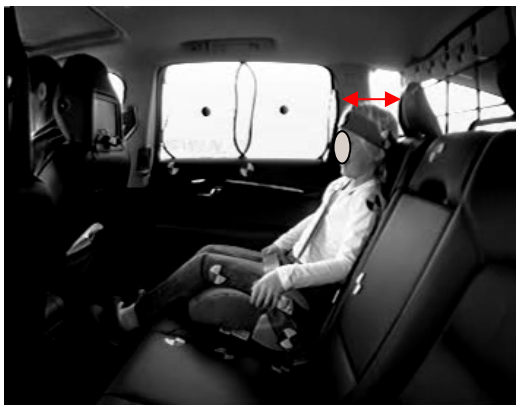
Figure 2a. Child 6 yo – 123 cm in rear seat of Volvo XC70 using booster cushion.
