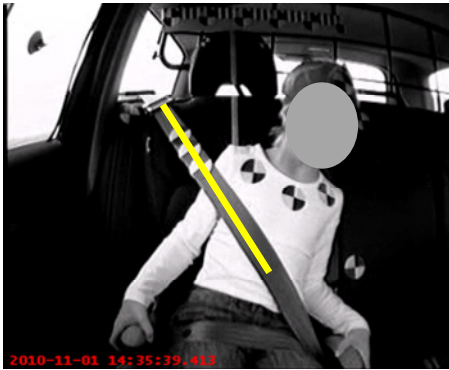
Figure 4a. Lateral inboard motion of a child during a swerving maneuver, using booster cushion (Bohman et al. 2011b)
